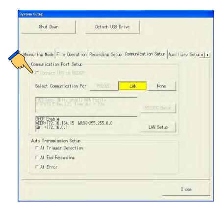
When the RA2300A is connected to UPS and a tick mark is added to the checkbox for "Connecting UPS to RS-232C", safety shutdown of the RA2300A can be made upon a power outage. After the power supply is resumed, startup is automatically made. If the power outage happens during recording or printing, the operation will be re-started.
