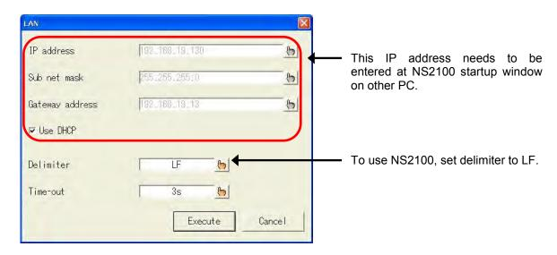
When DHCP is used, IP address is modified and as a consequence, the communication may be difficult to hold. In addition, DHCP is unusable in the case of peer-to-peer LAN connection. To solve the above problems, please input IP address without checking the box of "Use DHCP".
