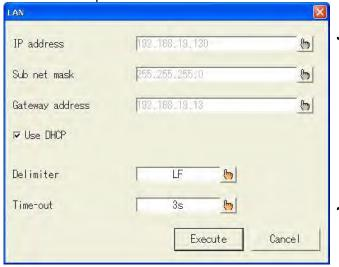
IP address, subnet mask, gateway address, delimiter, and timeout are set. Pressing a key opens the window for settings.
