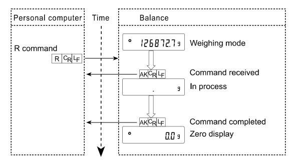
When a communication error has occurred due to external noise, or a parity error has occurred due to transmission error, the balance transmits an error code. In this case, send the command again.
