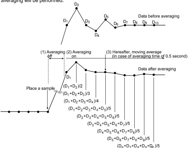
When a small amount of sample is weighed or is filled, the fluctuation of a weight value is too small to be beyond the selected range and the averaging operation is not disabled. Consequently moving averaging is always performed and it takes a longer time to reach the final weight value. Under such a situation, change the setting of "F |-b" to a smaller range. But please note that the smaller the range is, the more prone to external disturbance the value will become.
