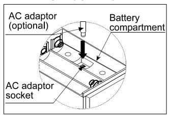
Plug the AC adapter to the AC adapter socket inside the battery compartment.
