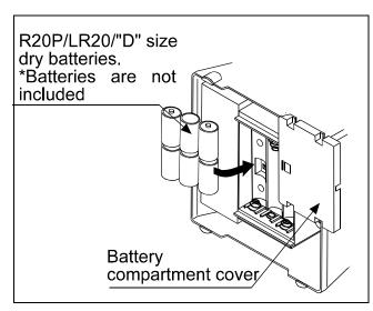
Remove the battery compartment cover and insert six batteries (R20P/LR20/D size) into the battery compartment, taking extreme care that the polarities plus and minus are observed.
