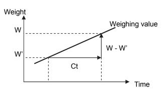
For flow rate calculation time Ct, select manual / automatic and set.
