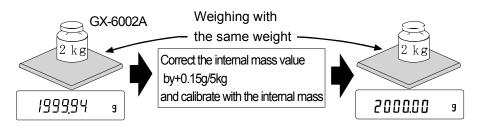
After performing one touch calibration, place the external weight on the balance and check the correction amount.
