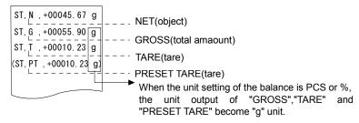
□ By using the "UFC function", output connection and order also can be set.
