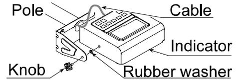
Step 2 Take the base unit and pole out, taking care that the load-cell cable is not pulled.
