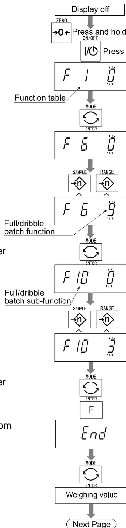
Step 8 Press the **MODE** switch to display the blinking HI (of the final value).
