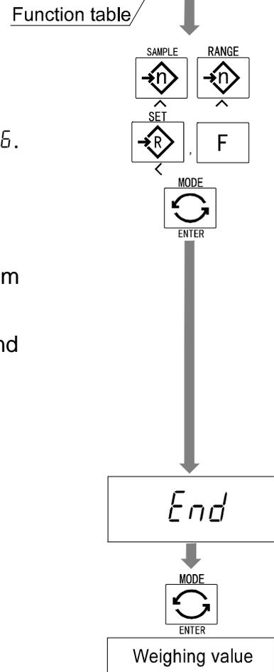
Step 3 Press the **ENTER** switch to return to the normal mode, when **End** is displayed.
