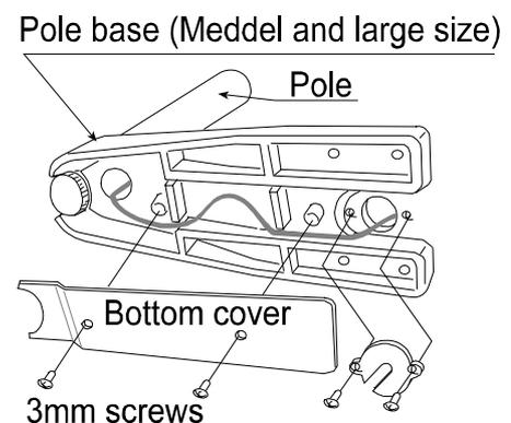
Step 8 Removing the pole base from the base unit, requires the following allen wrench.
