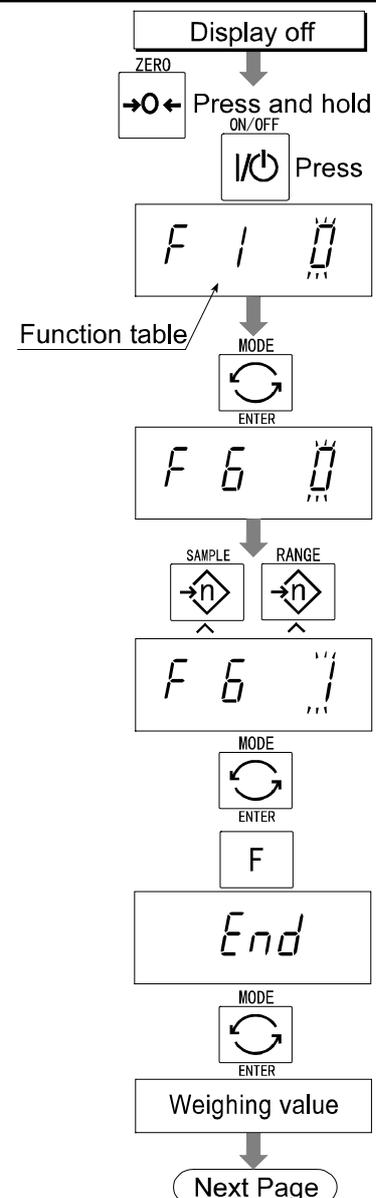
Step 6 If either of **F6 0**, **F6 2**, **F6 4**, **F6 6** has been selected, press the **SET** switch to use the comparator.
