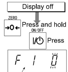
Step 2 Set parameters for each item using the following switches.
