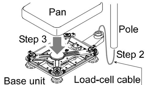
Step 3 Put the weighing pan on the base unit.
