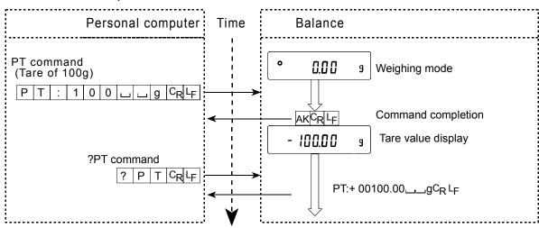
When a communication error has occurred due to external noise, or a parity error has occurred due to transmission error, the balance transmits an error code. In this case, send the command again.
