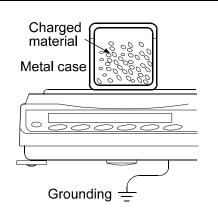
• This balance uses a strong magnet as part of the balance assembly, so please use caution when weighing magnetic materials such as iron. If there is a problem, use the underhook on the bottom of the balance to suspend the material away from the influence of the magnet.
