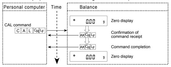
CAL command example (FX-i series: Calibration using an external weight)
