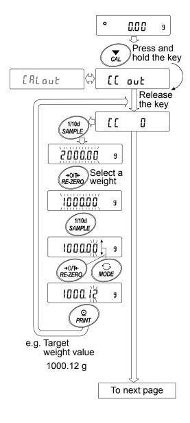
5 Confirm that there is nothing on the pan and press the PRINT key. The balance measures the zero point and displays the measured value. Do not allow vibration or drafts to affect the balance.
