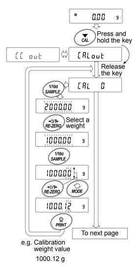
5 Confirm that there is nothing on the pan and press the PRINT key. The balance measures the zero point. Do not allow vibration or drafts to affect the balance.
