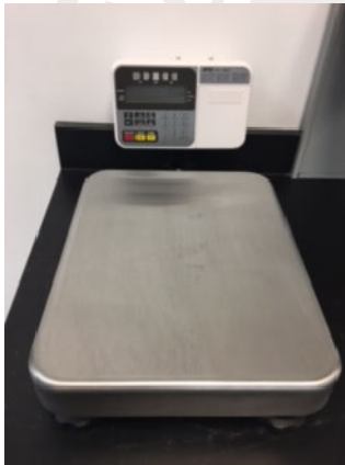
HV-60KC (60 kg) with remote cabled indicator
